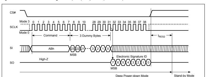
Figure 16. Read Electronic Signature (RES) Sequence (SPI Mode)
