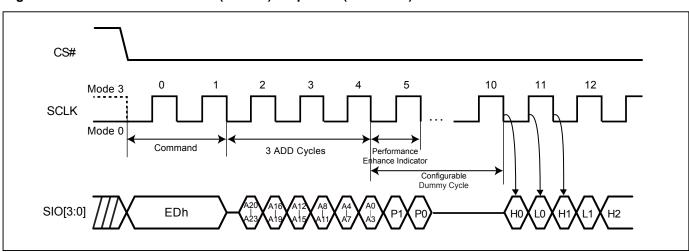
Figure 38. Fast Quad I/O DT Read (4DTRD) Sequence (QPI Mode)
