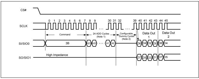
Figure 32. Dual Read Mode Sequence (SPI Mode only)
