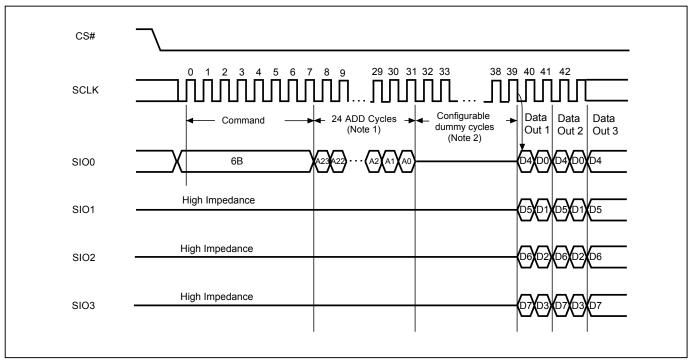
Figure 34. Quad Read Mode Seguence (SPI Mode only)
