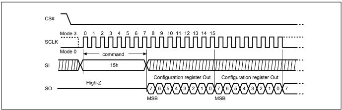
Figure 24. Read Configuration Register (RDCR) Sequence (QPI Mode)
