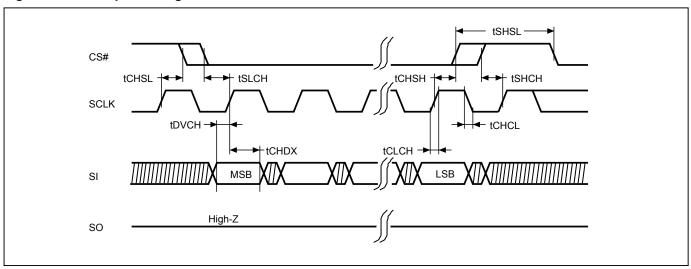
Figure 3. Serial Input Timing (DTR mode)
