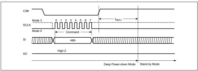
Figure 19. Release from Deep Power-down (RDP) Sequence (QPI Mode)
