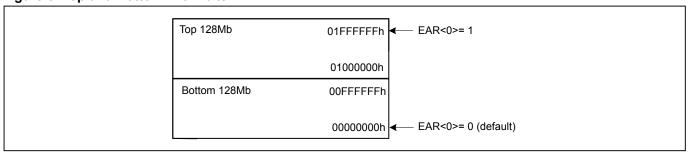
When under EAR mode, Read, Program, Erase operates in the selected segment by using 3-byte address mode.
