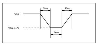
Figure 91. Maximum Positive Overshoot Waveform
