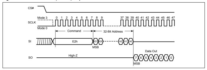
Figure 78. SPB Erase (ESSPB) Sequence
