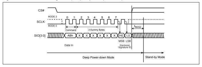
Figure 18. Release from Deep Power-down (RDP) Sequence (SPI Mode)
