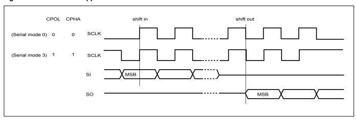
Figure 1. Serial Modes Supported
