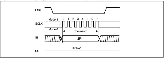
Figure 70. Write Security Register (WRSCUR) Sequence (QPI Mode)
