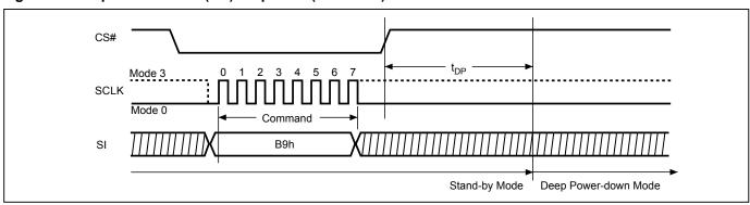
Figure 68. Deep Power-down (DP) Sequence (QPI Mode)
