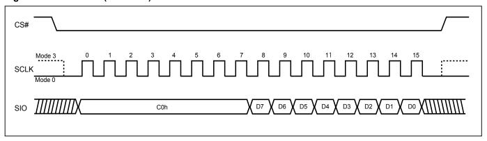
Figure 53. Burst Read (QPI Mode)
