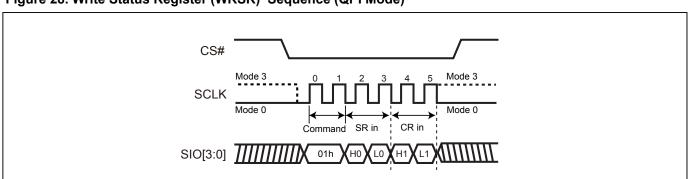
Figure 28. Write Status Register (WRSR) Sequence (QPI Mode)
