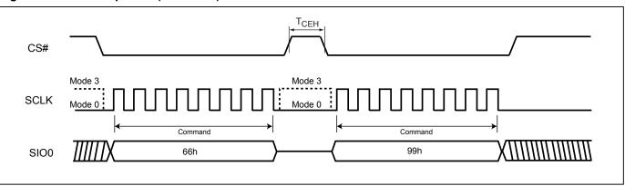
Figure 87. Reset Sequence (QPI mode)
