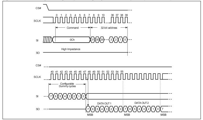
**Notes:** Configuration Dummy cycle numbers will be different depending on the bit6 & bit7 (DC0 & DC1) setting in configuration register.
