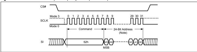
**Note:** Please note the address cycles above are based on 3-byte address mode. For 4-byte address mode, the address cycles will be increased.
