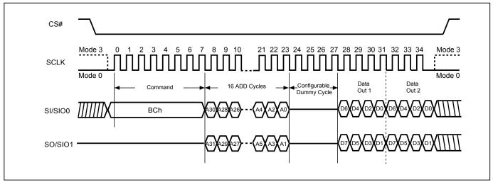
**Notes:** Configuration Dummy cycle numbers will be different depending on the bit6 & bit7 (DC0 & DC1) setting in configuration register.
