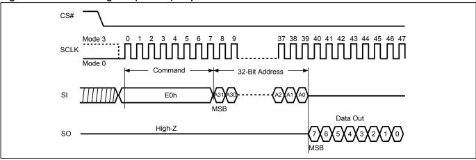
Figure 81. Write DPB Register (WRDPB) Sequence
