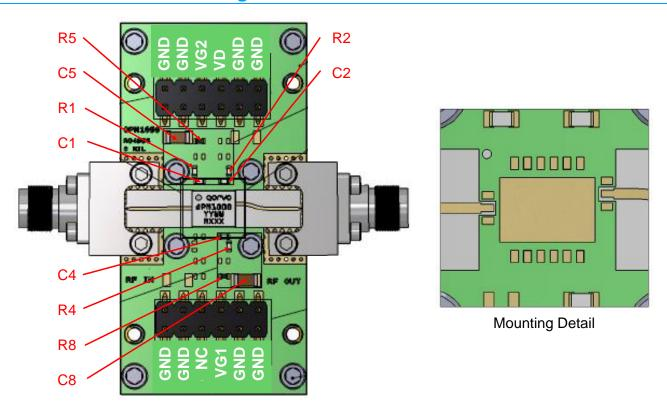
RF Layer is 0.008" thick Rogers Corp. RO40003C ( $\epsilon_r = 3.35$ ). Metal layers are 1.0 oz. copper. The microstrip line at the connector interface is optimized for the Southwest Microwave end launch connector 1092-01A-5.
