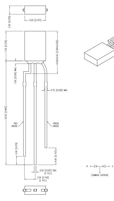
\*UNLESS OTHERWISE SPECIFIED TOLERANCES PER DECIMAL PRECISION ARE: X=±1 (±0.039), X.X=±0.5 (±0.020), X.XX=±0.25 (±0.010), X.XXX=±0.127 (±0.005). LEAD SIZE=±0.05 (±0.002), LEAD LENGTH=±0.75 (±0.030). MIN= +DECIMAL PRECISION MAX.= +0.00 -0.00 MAX.= +0.00
